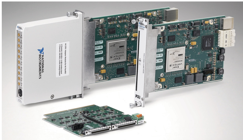
Figure 2 The FlexRIO-series FPGA modules use external adapter modules for I/O customization and are available in PXI and PXIe versions (courtesy National Instruments).
